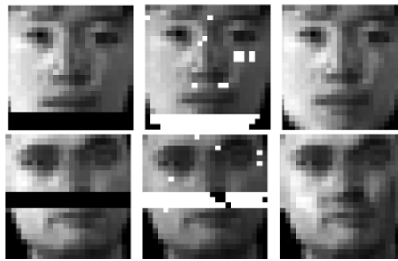
Fig. 5. This figure demonstrates the detection of the dead pixels, covering about 13% of the input image. Each row shows a distinct example drawn from the CMU-PIE dataset. Outliers detected by our method are marked as white pixels in the centre column, followed by the reconstructed images in the last column.
